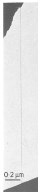
Figure 9 A thin (\text{SN})_x strand showing that they could be prepared for TEM observations without significant mechanical damage from twisting or bending. By rotating the strand 45^\circ about its axis it was shown not to be bent.
